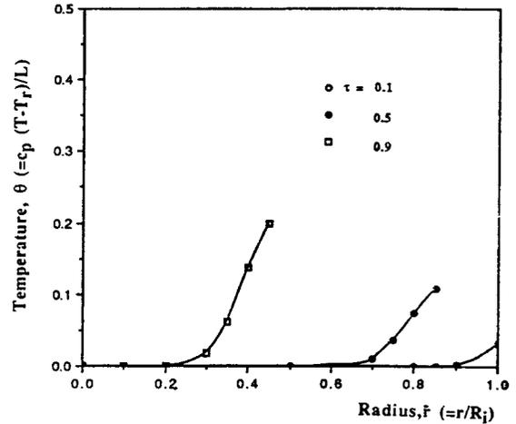
Fig. 6 Temperature profiles in vaporizing cloud for  $m_{1a} = 4.25$  ( $\tau = t/\tau_c$ , for octane cloud, table 2)
