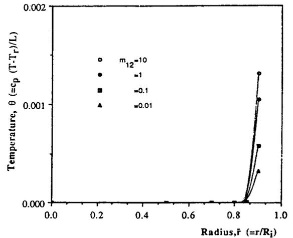
Fig. 7 Temperature profiles inside the cloud as a function of  $m_{12}$  at  $t/\tau_c = 0.1$  (for octane cloud, Table 2)
