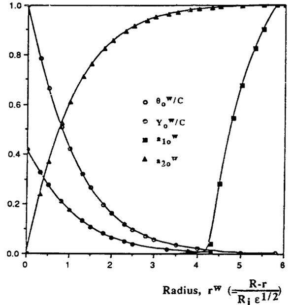
**Fig. 3** Structure of vaporization wave for  $m_{12}=0.01$  (for octane cloud, Table 2)
