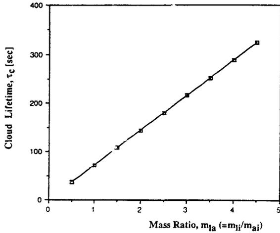
Fig. 5 Effect of mass ratio  $m_{1a}$  on cloud lifetime (for octane cloud, Table 2)
