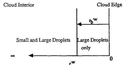
Fig. 2 Vaporization wave structure of bimodal sprays
