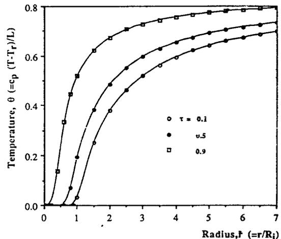
Fig. 8 Temperature profiles outside a vaporizing cloud for  $m_{1a} = 4.25$  and  $\theta_\infty = 1.00$  ( $\tau = t/\tau_c$ , for octane cloud, Table 2)
